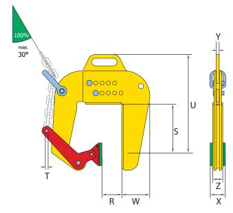
Terrier TBC / TBC-A lifting clamps must always be used in pairs (or per three clamps)
