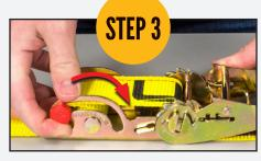
Move the red sliding bar to the "ADJUST" position.
