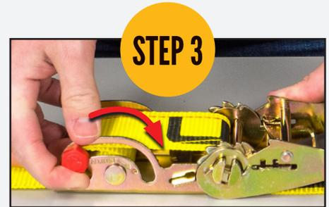
Move the red sliding bar to the **"ADJUST"** position.
