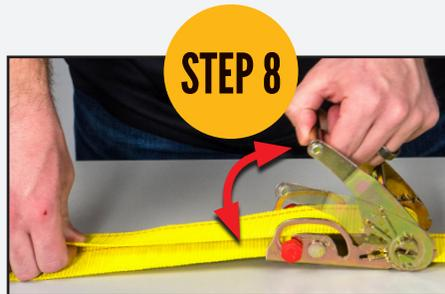
While holding excess webbing taut, ratchet the handle until load is secure.
