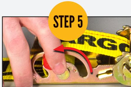
Move the red sliding bar to the **"LOCK"** position.
