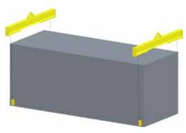
Straight setup Typically used with lift beam or spreader beam Used only on lower corners of the long slides
