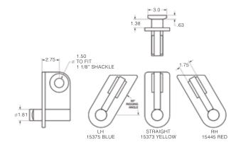
NOTE: Typical container lift will require 2 left and 2 right lugs. Or will require 4 straight lugs with appropriate spreader / lifting beam and rigging.
