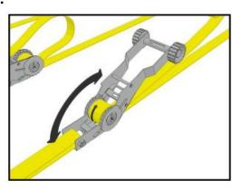
Attach the fixed end ratchet strap to the trailer or truck. Pull tight and ratchet down until the entire assembly is tight and your cargo is secure.
