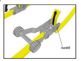
Feed the loose tail end of the strap through the ratchet mandrill.
