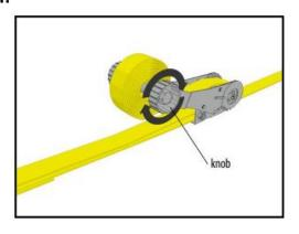
Roll up the ratchet strap by winding the knob. Tighten as far as you can, then twist the knob towards you to lock in place.
