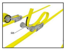
Take the tail end of the excess strap and insert into the spindle slot.
