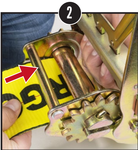
Feed loose end of long strap through ratchet mandrel, making sure webbing goes under the bar on the ratchet.
