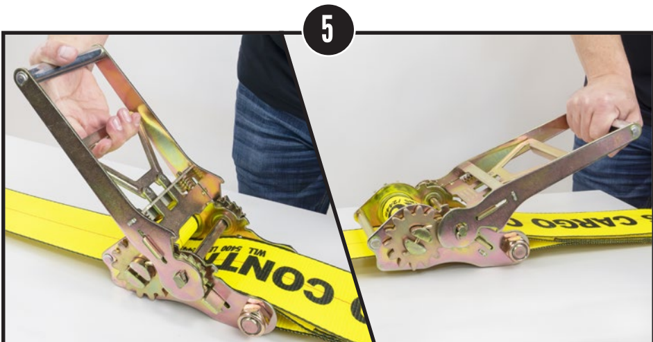
When ready to tighten the straps, squeeze the handle release and move the handle to the operating position. Move the handle back and forth to tighten the webbing.
