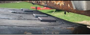
Trailer edge should contact upper end of 5<sup>th</sup> wheel Pads should be well under trailer
