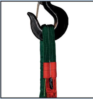
The Sling Tag should be placed 18-24 inches away from Connection Points.
