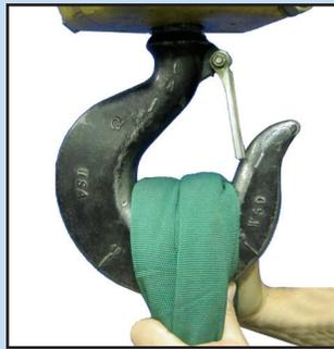
Squeeze both paths together to fit the Sling into the Connection Point.
