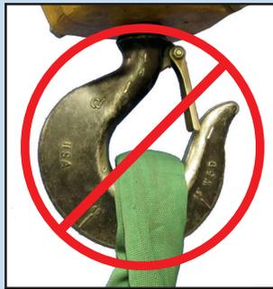
DO NOT fold one path over the other path to make the Sling "fit".
