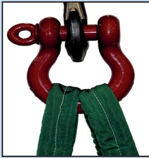
When placing multiple Twin-Path® Slings in hardware, place the Slings directly on top of each other or side by side. DO NOT stair-step paths partially over each other.
