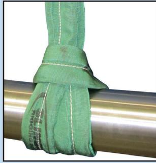
Make sure the paths of the Sling are smooth in the bite of the choker hitch without twisting.
