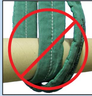
When rigging a choker or basket hitch, DO NOT pull slack out of the Sling with the crane.
