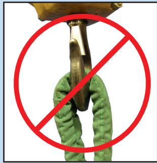
Keep folds and wrinkles off the hook, hardware and/or load.
