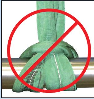
DO NOT allow the Sling to roll over itself and twist at the bite of the choker hitch.
