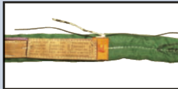
TATTLE TAIL MISSING (Sling fails inspection)
