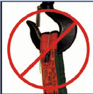
DO NOT place the sling tag in the hook, shackle or connection hardware.
