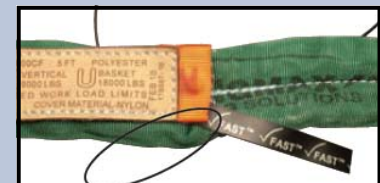
EWI MISSING (Sling fails ✓Check Fast® Criteria)
