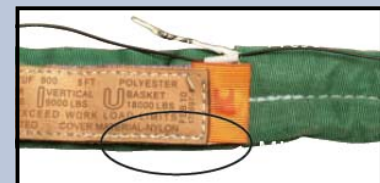
TATTLE TAIL MISSING (Sling fails)
