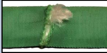
CUT OR DAMAGED YARNS
