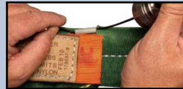
FIBER OPTIC (Lack of light transfer—Sling Fails)
