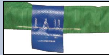
MISSING OR ILLEGIBLE TAG
