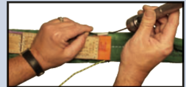
FIBER OPTIC-No Light Transfer (Sling fails inspection)
