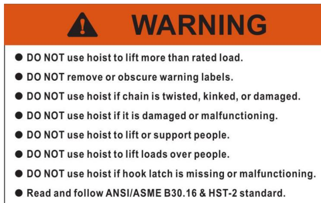
Figure 1 Warning Label Attached to Chain Hoist (shown larger for legibility)
