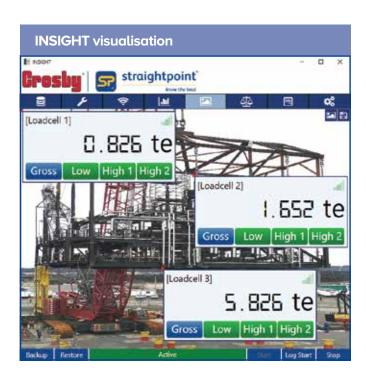
INSIGHT software, supplied with an SW-D USB wireless dongle, allows connection of up to 126 Straightpoint wireless load cells simultaneously onto any Windows tablet or laptop.
