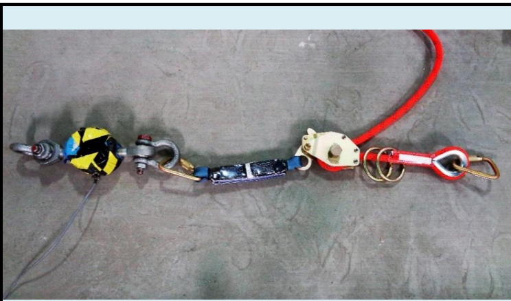
Figure 3: Kernmantle HLL Test Configuration Mockup
