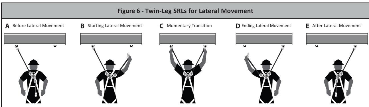
Avoid sudden or quick movements during the normal work operation, as this may cause the SRL pawl system to engage and possibly cause loss of balance, which may cause injury or death. If a fall occurs, the pawl system will engage and lock the lifeline. The EA will deploy to arrest the fall and limit arrest forces on the user.
