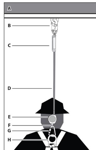
**5.2 Single SRL Installation to Anchorage:** SRLs with large opening rebar hooks for leg-end connectors are not permitted for this type of installation due to incompatibility. See Section 4.2 Installation for Single-leg configuration of the DuraTech Mini to an anchorage or anchorage connector follows the steps listed below. :
