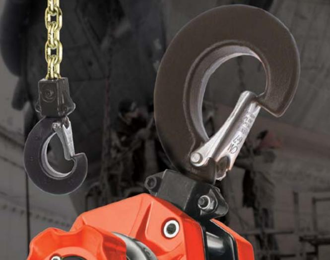
With a blunt tip and the ability to point load, these hooks are ideal for positioning steel plates and figures during welding. They are used in common applications like shipbuilding, metal fabrication and many other industries. Optional on 1-1/2 and 3 Ton CM Tornado 360° units, these hooks are forged from 8630 quenched and tempered alloy in the USA and have a 4:1 design factor.
