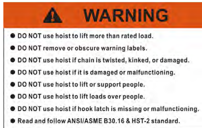
Figure 1 Warning Label Attached to Chain Hoist
