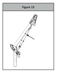
The Davit Arm is a dynamic anchorage system that will vary in its performance depending upon the configured offset. Care should be taken to understand the capacity of the system and anchorage strength requirements; see Figure 14 for the load ratings for the 24" to 44" Offset Davit Arm.
