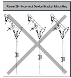
To attach a winch or 3-Way to the Davit Device Receiver Bracket, place the notch in the device side bracket over the bottom bar of the bracket as shown in Figure 30. Rotate to align the upper holes, see Figure 31. Insert the provided detent pin, see Figure 32.
